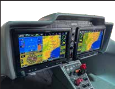
Central console with "Dual GARMIN G3X Displays"
