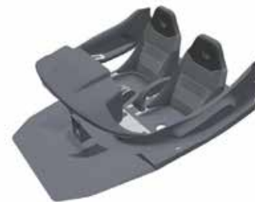
Side arm rest with niches for BOSE headset controls
